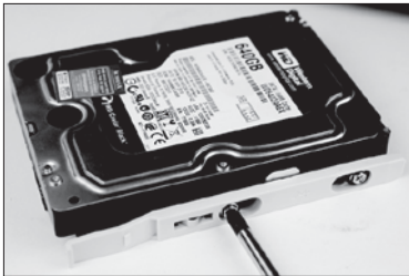
① Install the Anti-Vibration HDD Guides to the left and right sides of the 3.5" HDD.
